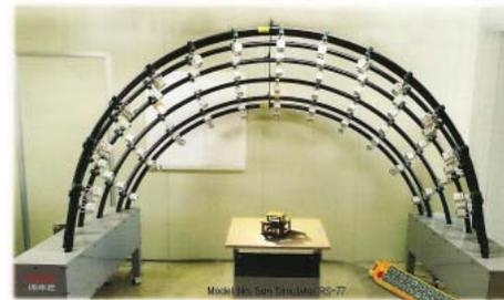
Fig. 2 The Sun Simulator with hand held remote control unit. —구신 리우
