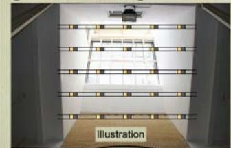
A "flux-net" is a sparse mesh of small rectangles of paper strung across a building aperture. Half of each rectangle has an opaque patch on the upper side.
