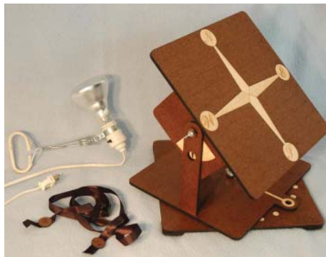
Finely crafted personal table-top heliodons can be constructed from readily available materials.
