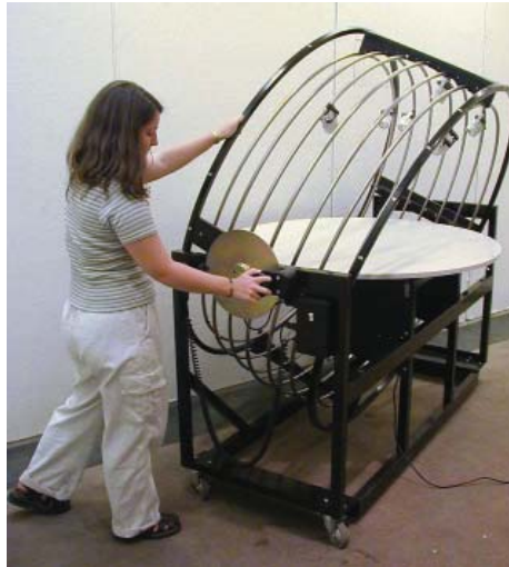
A student demonstrates the ease of use of the full-scale, conceptually clear “sun-emulator” heliodon.
