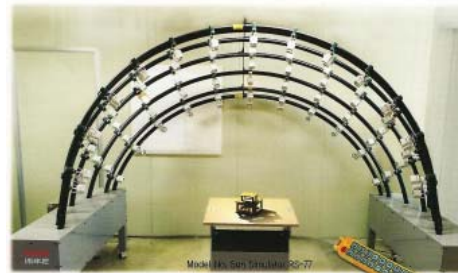
Fig. 2 The Sun Simulator with hand held remote control unit. —구신 리우 The multi-sun path “sun-simulator” heliodon.
