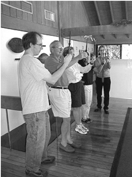
Fig. 2. From one deck to another, instantaneous velocity measurements were taken using hot-wire anemometers.
