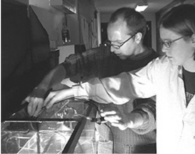
Fig. 5. Placing the copper wire leads through the base of the model while submerging it into the tank of water required several sets of hands.
