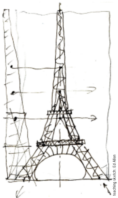
The Eiffel Tower was designed from force diagrams.
